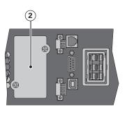
It is not necessary to shutdown the UPS before installing a communication card.
